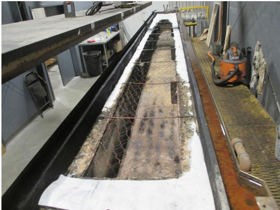
Photo No. 4 Post-Test Unexposed Side
