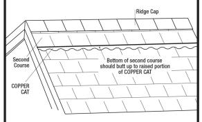
From left, use a roofing flat bar to lift bottom of 2nd course. Slide a COPPER CAT strip under 3/4" to where bottom of shingle butts up to COPPER CAT'S raised portion, nail down, repeat to end.
